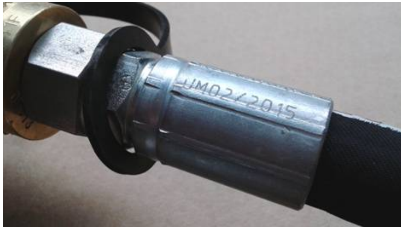
Fig.2 - Example of date of manufacture engraved on the hose fitting (UMmm/yyyy)
