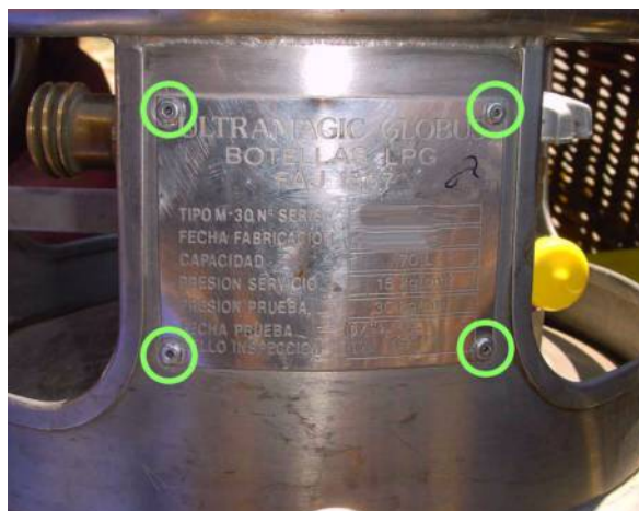
Fig.1 - Cylinder ID plate fitted with Alu-rivets. Content and format of the ID plate may differ.
